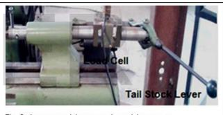
Fig. 2. Arrangement for measuring axial pressure
