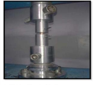
Fig. 6. Collet used for mechanical testing.
